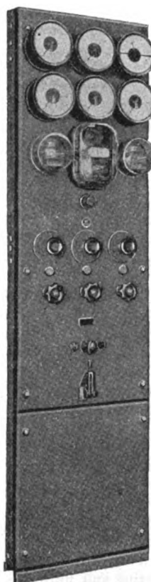
FIG. 2—SWITCHBOARD WITH CONTROL EQUIPMENT
